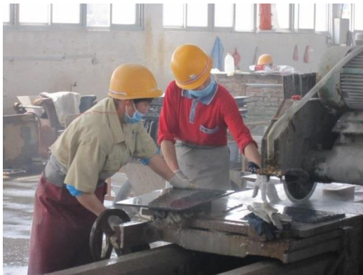
工人穿戴个人防护设备，但防尘面罩不是 FFP2 面罩，且没有盖住鼻子 Workers are wearing PPE but dust masks are not FFP2 and are not covering the nose.
